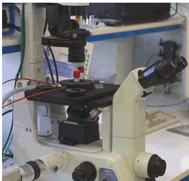
Figure 3. Quiescent thermostated cell by Peltier effect placed under a microscope equipped with a camera.
